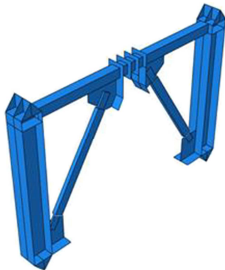
Figure 4. BRBF with shear link [26].
