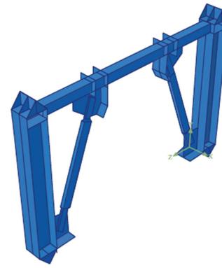
Figure 6. BRBF with moment link [25].
