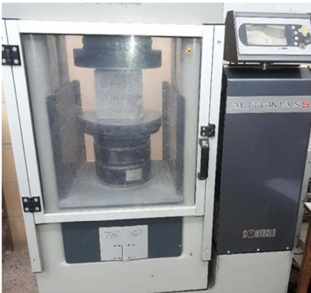
Figure 5. Compressive strength test.
