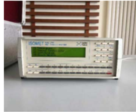
Figure 9. ISOMET2104 heat transfer analyzer.
